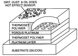
**TEMPERATURE & HUMIDITY EFFECTS:** The output of all absorption based humidity sensors (capacitive, bulk resistive, conductive film, etc.) are affected by both temperature and %RH. Because of this, temperature compensation is used in applications which call for either higher accuracy or wider operating temperature ranges.
