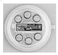
The HIH-3602-C incorporates a RHIC humidity sensor, a  $1000\Omega$  platinum RTD and anti-static protection in a single TO-5 can.
