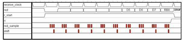
Fig. 8-6: Receive modes 2 and 3 for Serial 0
