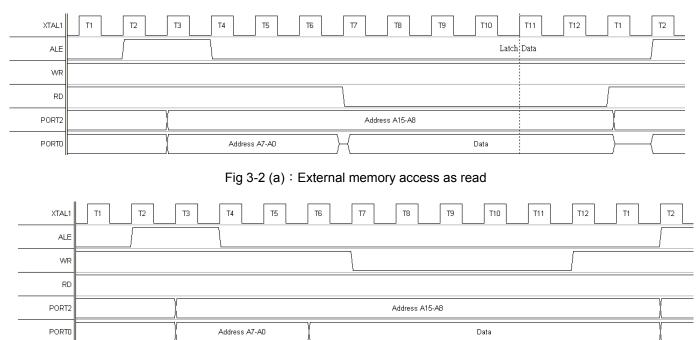
Fig 3-2 (b) : External memory access as write
