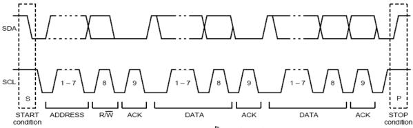
Fig. 13-2: RW bit in the 8<sup>th</sup> bit after IIC address
