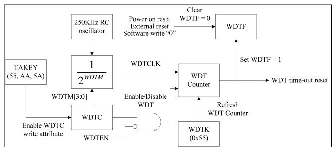
Fig. 9-1: Watchdog timer block diagram
