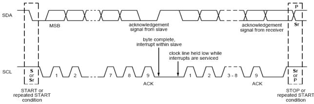
Fig. 13-1: Acknowledgement bit in the 9<sup>th</sup> bit of a byte transmission
