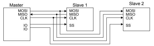
Fig. 14-1: SPI signals between master and slave devices
