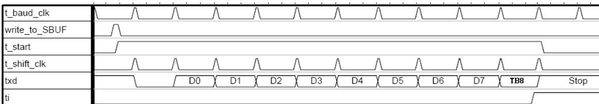
Fig. 8-5: Transmit modes 2 and 3 for Serial 0
