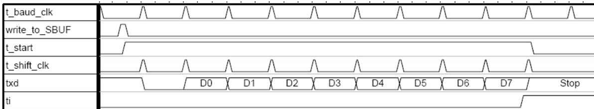
Fig. 8-3: Transmit mode 1 for Serial 0
