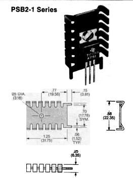
Dimensions are for reference use only. Contact IERC for dimensions with tolerances or standard part drawings.
