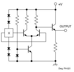
Early Linear Ratiometric Sensor Using Single Hall Element
