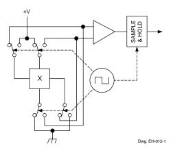
Electronically Rotated Sensor to Cancel Effects of Strain
